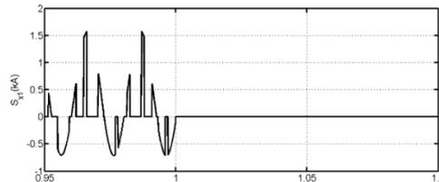
(e) Sample of current waveform in switch  $S_{x1}$  (first cell of phase a upper arm)
