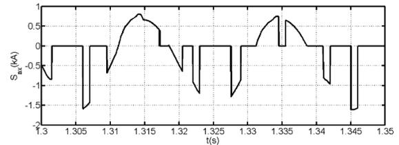
(f) Sample of current waveform in switch  $S_{x1}$  (first cell of phase a upper arm)
