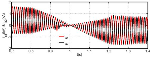
(c) Samples of the upper and lower arm currents ( $i_{a1}$  and  $i_{a2}$  of phase a)
