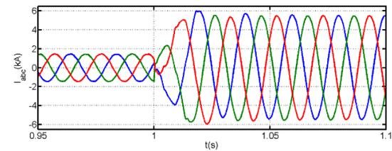
(a) Current waveforms MMC1 injects into PCC<sub>1</sub>
