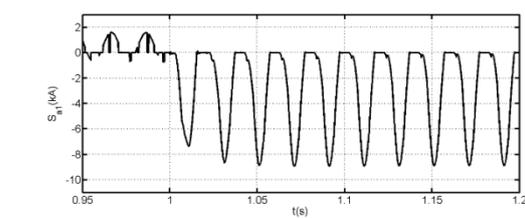
(d) Sample of current waveform in switch  $S_{a1}$  (first cell of phase a upper arm)
