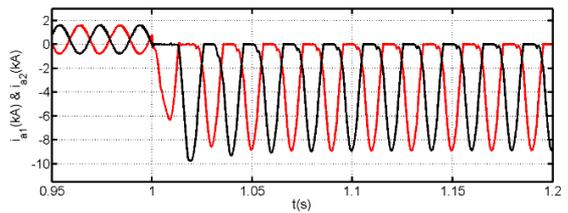
(b) Samples of the upper and lower arm currents ( $i_{a1}$  and  $i_{a2}$  of phase a)
