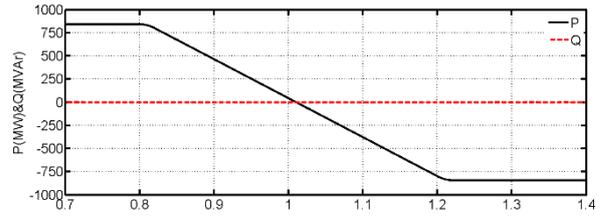
(b) Active and reactive power converter station exchanges with ac network at PCC<sub>1</sub>
