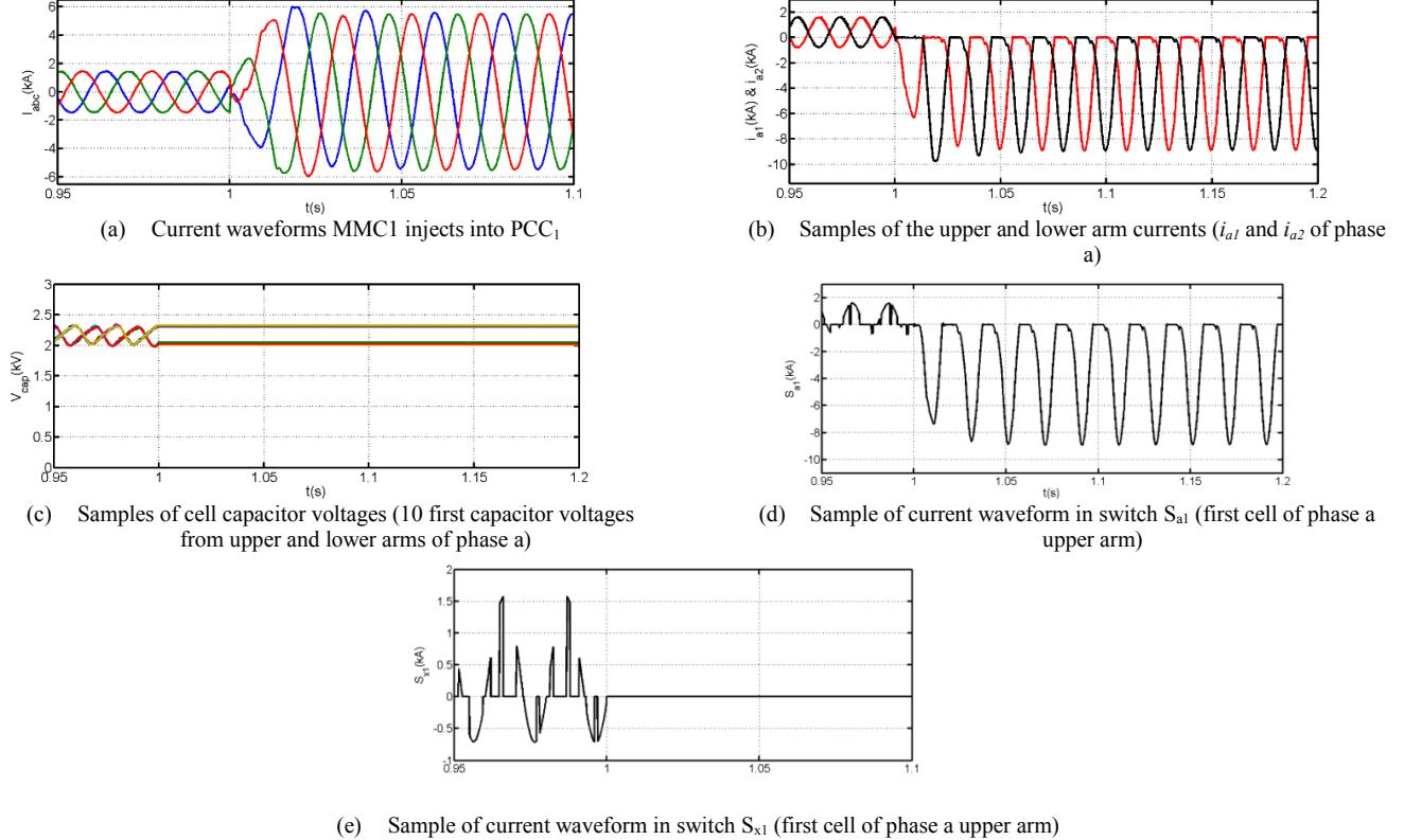
Fig. 6: Waveforms illustrating the capabilities of the proposed switching function based MMC model in capturing detailed behaviour of MMC during dc fault
