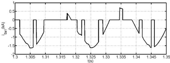
(e) Sample of current waveform in switch  $S_{a1}$  (first cell of phase a upper arm)
