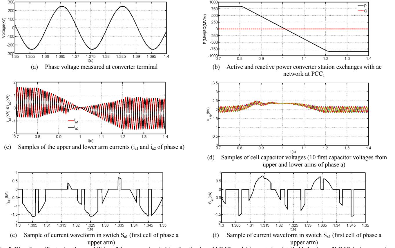
Fig. 5: Waveforms illustrating the capabilities of the proposed switching function based MMC model in capturing detailed behaviour of MMC during normal operation
