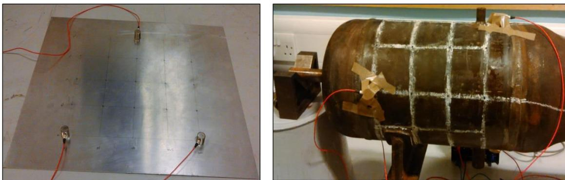
**Figure 1.** Experimental specimens for source location experiment
