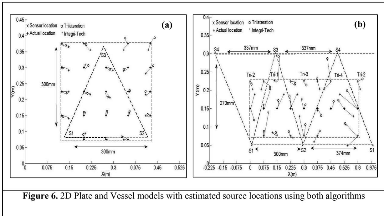
**Figure 6.** 2D Plate and Vessel models with estimated source locations using both algorithms
