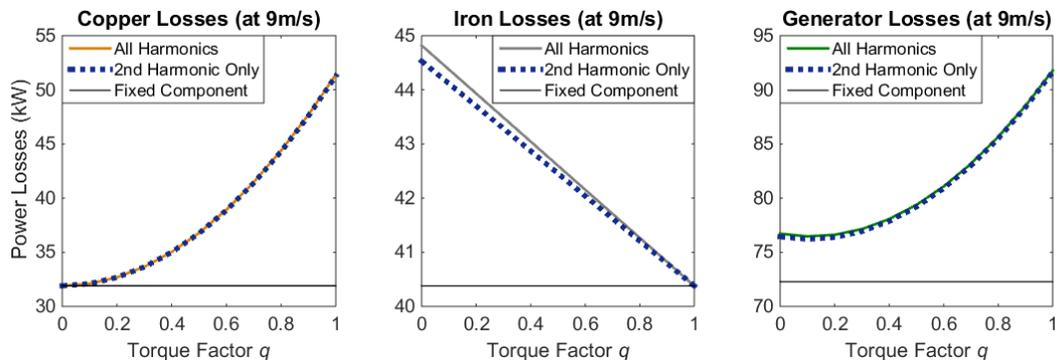
Fig. 3. Generator Losses (at 9m/s) considering (a) 2nd Harmonic only, (b) All Harmonics
