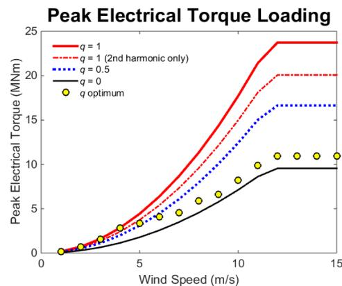
**Fig. 6.** Peak Electrical Torque at different wind speeds for different  $q$  strategies
