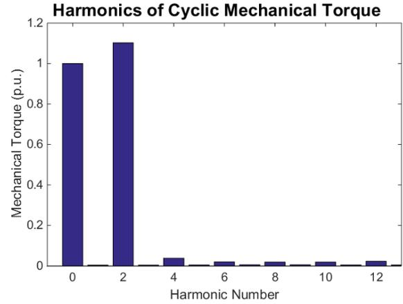
Fig. 2. Harmonic Components of Cyclic Mechanical Torque Loading
