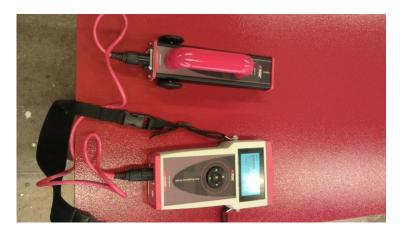
Figure 8: TQC Hull Roughness Gauge.
