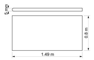
Figure 1: Dimensions of the flat plates.
