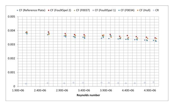
Figure 11: Frictional resistance coefficients of all test surfaces together with C<sub>R</sub> values.
