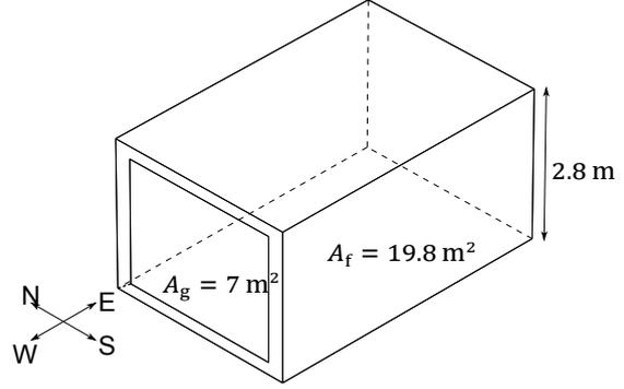
Figure 2: Wire frame drawing of office zone
