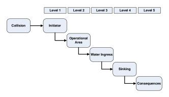
Figure 2 High-level event sequence for collision casualties of passenger ship
