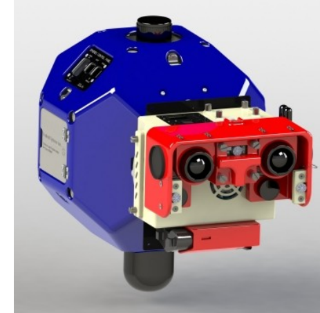
SPHERES with VERTIGO vision system (Credit: MIT Space Systems Laboratory)
