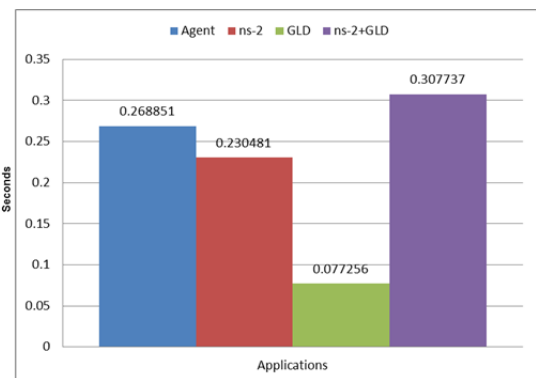
Fig. 4. Average execution time for 1000 test cases of ns-2, GLD, Agent and combined average time of ns-2 with GLD
