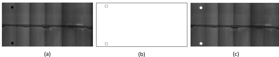
**Figure 3 Trepanned hole detection using Hough Transform for circle detection – (a) original image (b) Binary result of circle detection algorithm (c) circles detected overlaid on original and filled in**
