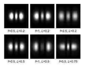
FIG. 8: Density patterns for the output of different configurations of resonator, calculated for g=0. f represents the focal time of the lens pulse, L the time between subsequent pulses (both in dimensionless units). For the particular choice of loss-pulse shape, the loss per period of the light-pulse resonator for these eigenmodes is, from top left to bottom right, 1.8%, 1.3%, 5.9%, 4.4%, 10.2%, and 9.7%.
