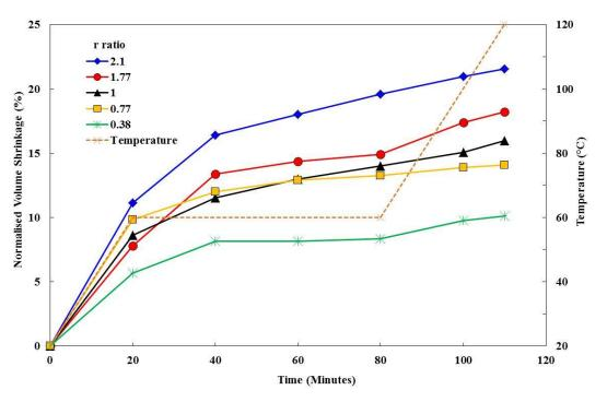
Figure 3. Normalised volumetric shrinkage of microbond droplets during curing
