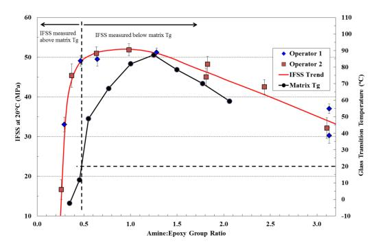
Figure 2. IFSS and matrix Tg versus amine:epoxy group ratio in matrix
