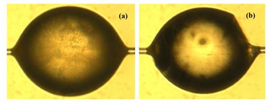
Figure 4. Optical micrographs of epoxy droplet on glass fibre. (a) before cure. (b) after cure
