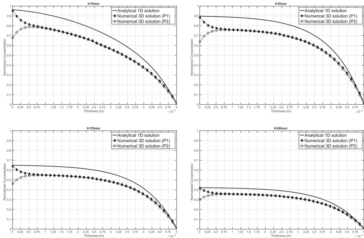
Fig. 2. Updated results for the case of halved strut thickness and separation. Convection dominated regime. This replaces Fig. 7 of the original paper.
