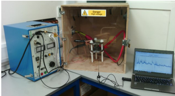
Fig. 2. RTL-SDR dongle connected to the laptop via USB port.
