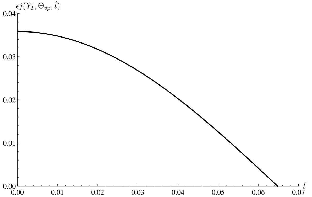
Figure 15: Graph of the radial perturbation  $j(Y_I, \Theta_{op}, \hat{t})$  versus the nondimensionalised time for  $\mu = 20\text{MPa}$ ,  $\nu = 0.49$ ,  $\beta = 24.5$ , an initial thickness of  $Y_O - Y_I = 0.02$ , an opening angle of  $\pi - \Theta_{op} = \pi/36$  and a matching boundary condition at  $\Theta_s = \pi/45$ . This is calculated using equations (142), (144), (145), (151) and (155).
