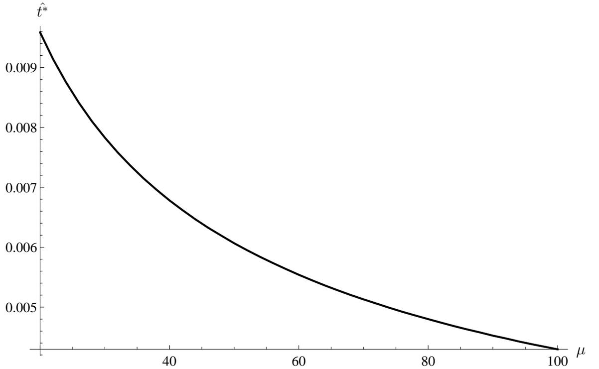
Figure 11: Graph of the nondimensionalised collapse time for the collapse phase of the shell versus a range of shear modulus values for  $\nu = 0.49$ ,  $\beta = 24.5$ , an initial thickness of  $Y_O - Y_I = 0.02$ , an opening angle of  $\pi - \Theta_{op} = \pi/36$  and a matching boundary condition at  $\Theta_s = \pi/45$ . This is calculated using equations (165), (166), (167), (168) and (169).
