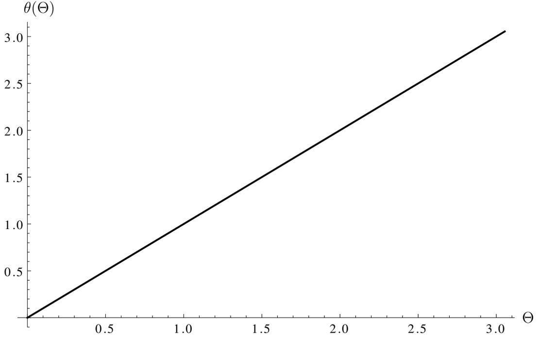
Figure 5: Graph of  $\theta(\Theta)$  for an open shell versus the reference angle,  $\Theta$ , for a nondimensionalised stress load of  $\hat{p} = 0.0002$  where  $\mu = 20\text{MPa}$ ,  $\nu = 0.49$ ,  $\beta = 24.5$  and an initial thickness of  $Y_O - Y_I = 0.02$  for an opening angle of  $\pi - \Theta_{op} = \pi/36$  and a matching boundary condition at  $\Theta_s = \pi/45$ . This is calculated using equation (118).
