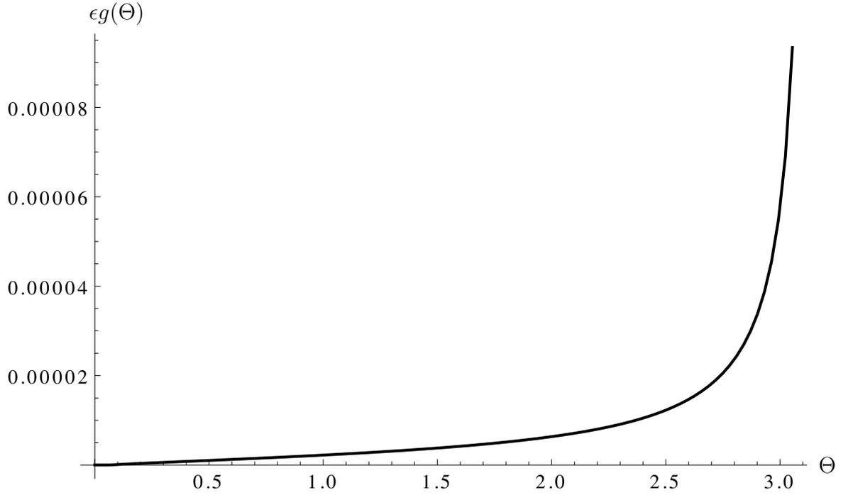
Figure 4: Graph of the angular perturbation for an open shell versus the reference angle for a nondimensionalised hoop stress load of  $\hat{p} = 0.0002$  where  $\mu = 20\text{MPa}$ ,  $\nu = 0.49$ ,  $\beta = 24.5$  and an initial thickness of  $Y_O - Y_I = 0.02$  for an opening angle of  $\pi - \Theta_{op} = \pi/36$  and a matching boundary condition given at  $\Theta_s = \pi/45$ . This is calculated using equation (118).
