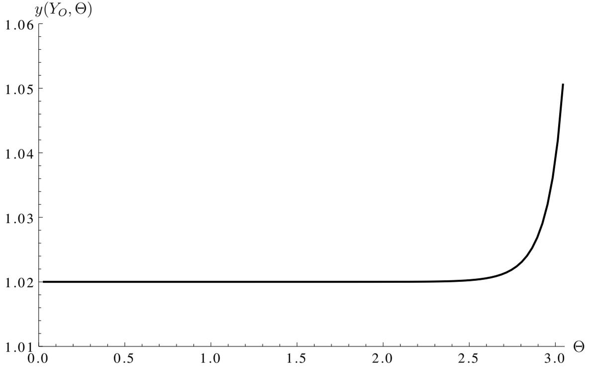
Figure 7: Graph of the nondimensionalised radius in the current configuration  $y(Y, \Theta)$  versus  $\Theta$  for a nondimensionalised stress load  $\hat{p} = 0.0002$  where  $\mu = 20\text{MPa}$ ,  $\nu = 0.49$ ,  $\beta = 24.5$  and an initial thickness of  $Y_O - Y_I = 0.02$  for an opening angle of  $\pi - \Theta_{op} = \pi/36$  and a matching boundary condition at  $\Theta_s = \pi/45$ . This is calculated using equations (122) and (129).
