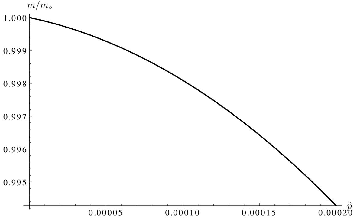
Figure 9: Graph of the normalised mass  $m/m_o$  for a series of nondimensionalised stresses loads up to  $\hat{p} = 0.0002$  where  $\mu = 20\text{MPa}$ ,  $\nu = 0.49$ ,  $\beta = 24.5$  and an initial thickness of  $Y_O - Y_I = 0.02$  for an opening angle of  $\pi - \Theta_{op} = \pi/36$  and a matching boundary condition at  $\Theta_s = \pi/45$ . This is calculated using equations (74), (122) and (129).
