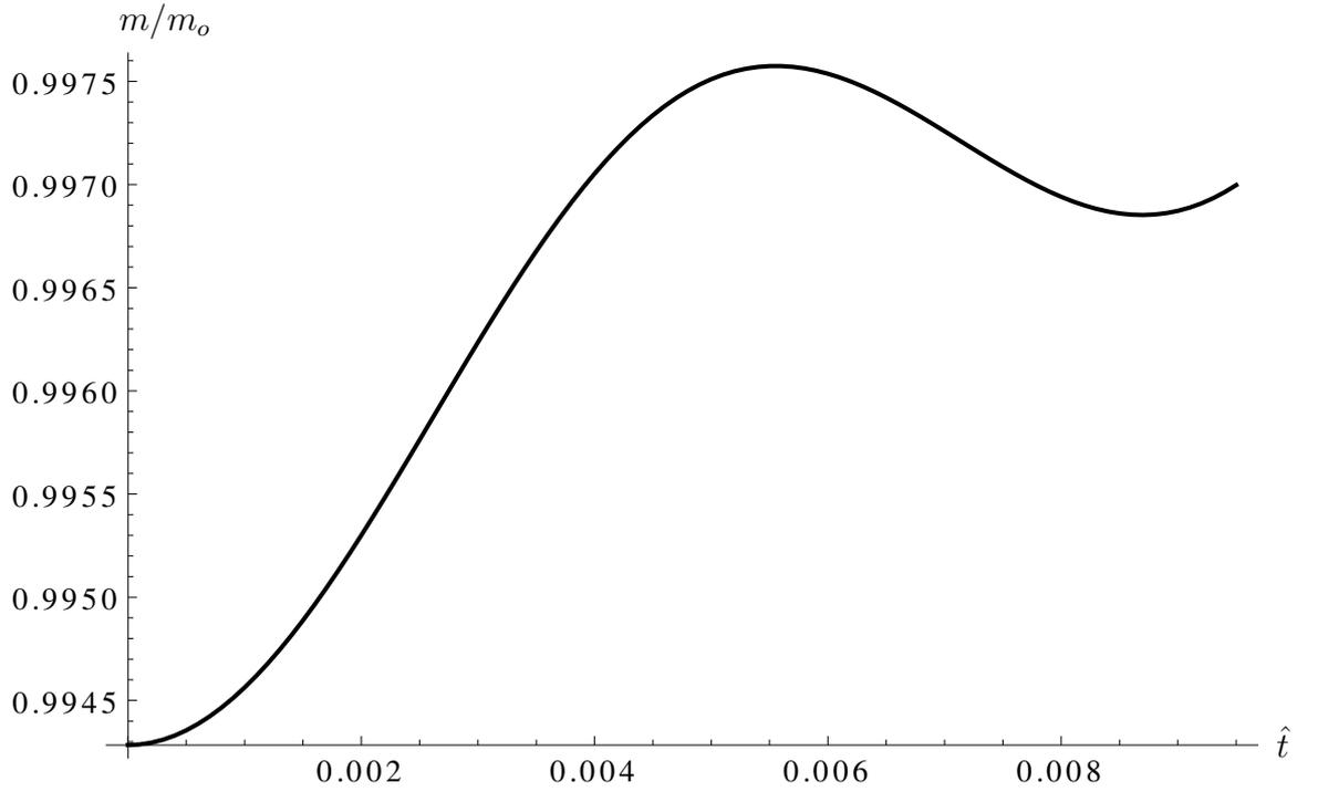
Figure 14: Graph of the normalised mass  $m/m_o$  of a stressed, collapsing shell where  $\mu = 20\text{MPa}$ ,  $\nu = 0.49$ ,  $\beta = 24.5$  and an initial thickness of  $Y_O - Y_I = 0.02$  for an opening angle of  $\pi - \Theta_{op} = \pi/36$  and a matching boundary condition at  $\Theta_s = \pi/45$ . This is calculated using equations (165) to (169).
