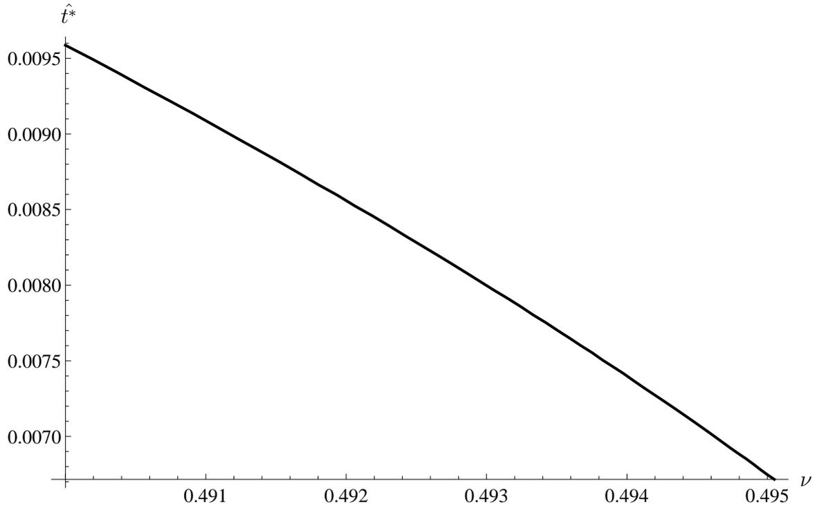
Figure 12: Graph of the nondimensionalised collapse time versus a range of Poisson ratios for  $\mu = 20\text{MPa}$ , an opening angle of  $\pi - \Theta_{op} = \pi/36$  and a matching boundary condition at  $\Theta_s = \pi/45$ . This is calculated using equations (165), (166), (167), (168) and (169).
