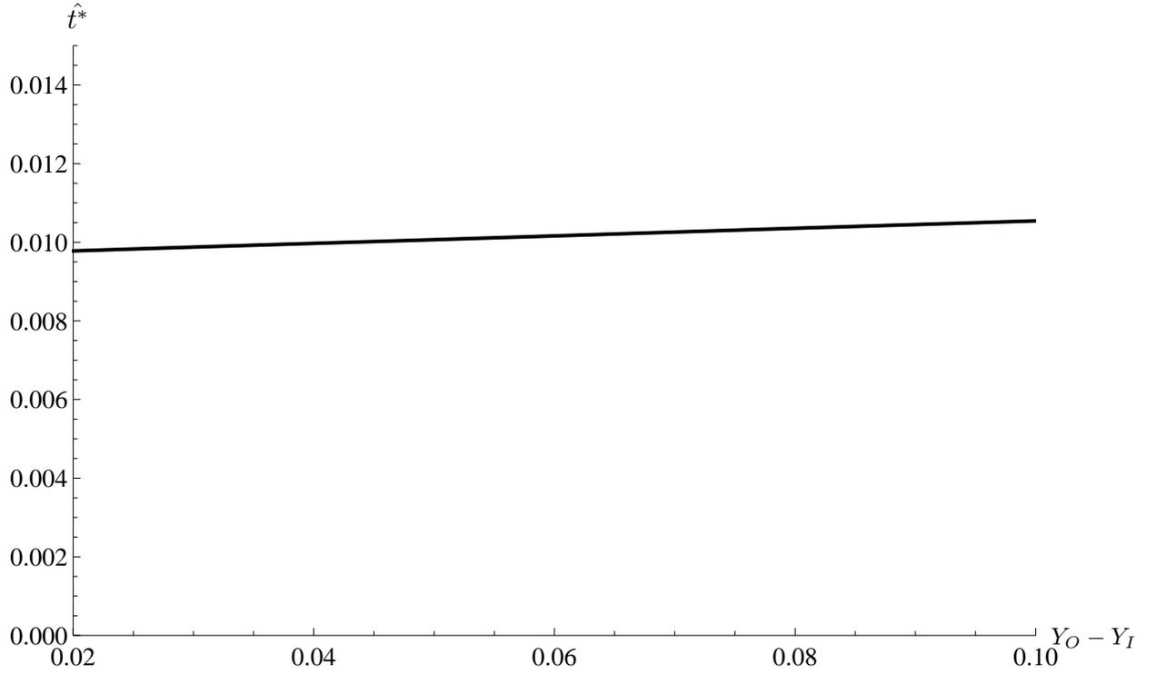
Figure 13: Graph of the nondimensionalised collapse time  $\hat{t}^*$  versus a range of nondimensionalised stress free shell thicknesses ranging from  $Y_O - Y_I = 0.02$  to  $0.10$  for  $\mu = 20\text{MPa}$ ,  $\nu = 0.49$ ,  $\beta = 24.5$ , an opening angle of  $\pi - \Theta_{op} = \pi/36$  and a matching boundary condition at  $\Theta_s = \pi/45$ . This is calculated using equations (165), (166), (167), (168) and (169).
