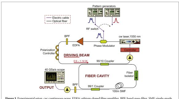
Figure 3. Experimental setup. cw: continuous-wave, EDFA: erbium-doped fibre amplifier, BPF: band-pass-filter, SMF: single-mode fibre.
