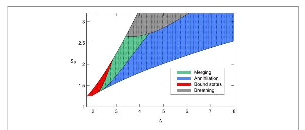
**Figure 2.** Results from numerical simulations illustrating the outcome of LDS interactions as a function of driving frequency  $\Delta$  and strength  $S_0$  for  $\phi(0)=0.5$  rad, and  $x_0=30$ . Each solid dot represents a distinct simulation. No LDSs exist in the white-colour coded area.
