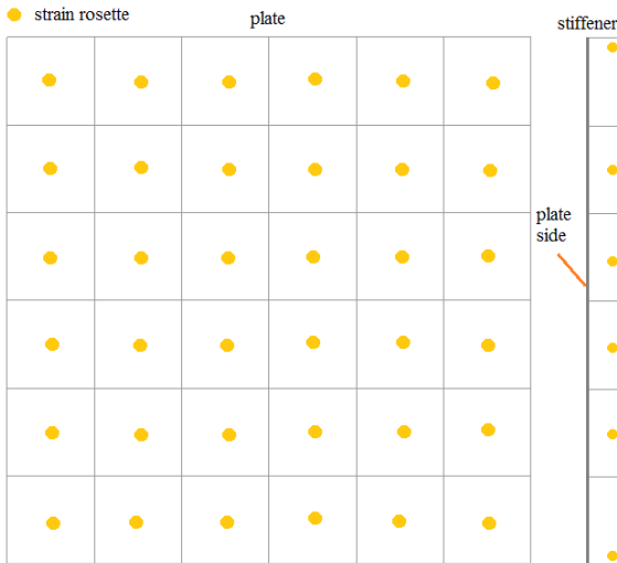
Figure 12. Approximate locations of 96x2 strain rosettes on stiffened plate discretized by 96 iQS4 elements.
