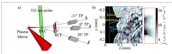
**Figure 1.** (a) Experimental set-up. (b) Probe shadowgraphy at t=250 ps after the interaction together with phase map, in units of the line density integral, from simultaneous interferometry (red box) for  $d_0=100$  nm, LP. The yellow line indicates the initial position of the rear surface measured before the shot.
