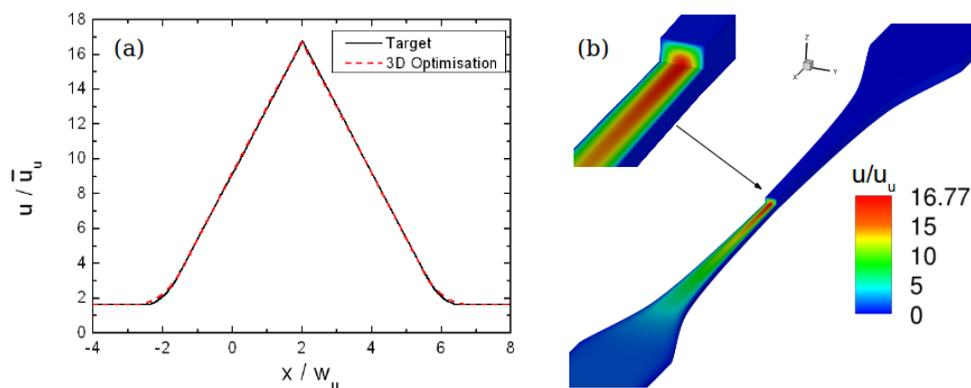
**Figure 1.** Velocity profile of the optimised solution versus the desired target profile, along the centreline of the channel for a Newtonian fluid (a) and dimensionless velocity contours for an optimised 3D converging geometry (b) with  $\epsilon_H = 2$ .
