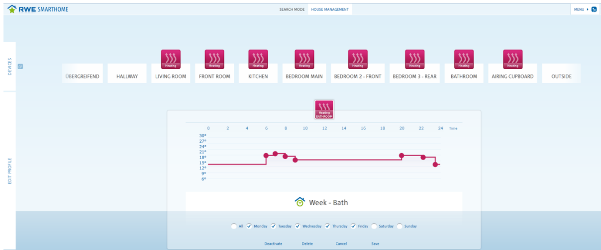
Figure 3: Screenshot of House19's weekday 'Bath' profile (taken on 9/12/14, 2.5mths after installation)
