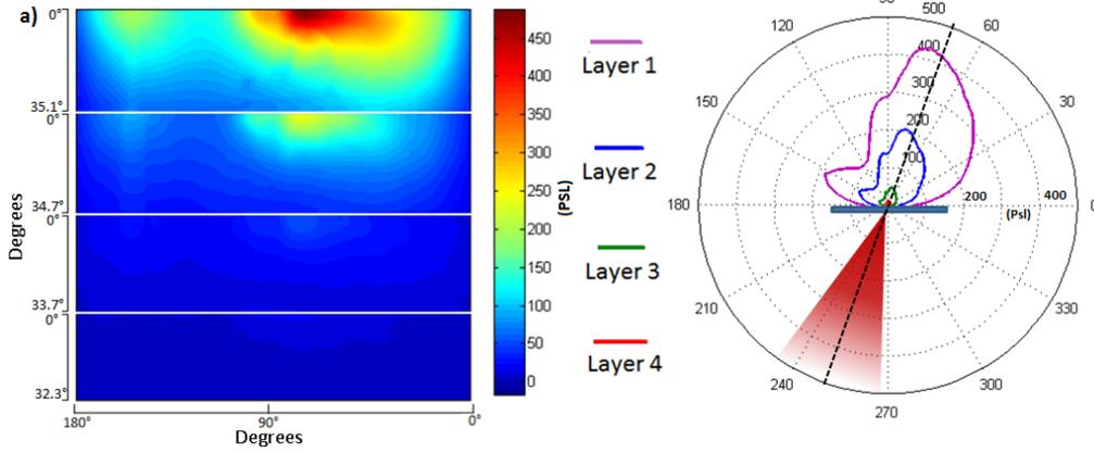
FIGURE 4. (a) PSL signal from the remapped layers of IP between the Fe filtering from a 140J shot onto a 100um Cu target. (b) a polar plot of the data. The peak emission appears to be close to laser axis.
