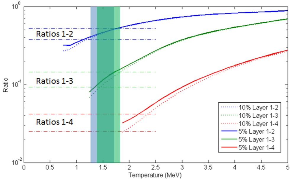
FIGURE 6. Ratios of layer 1 to each sequential layers from a relativistic electron beam passing through a 100um Cu target with an upper limit of the escaping electron fraction of 10% and a lower limit of 5%. The data, represented by the horizontal lines, intersects the simulated ratios which is shown by the shaded regions. The overlapping area for this shaded region lays between the temperatures of 1.4 and 1.7 MeV. For the ratio 1-4, the ratio is outside the working range of the diagnostic.
