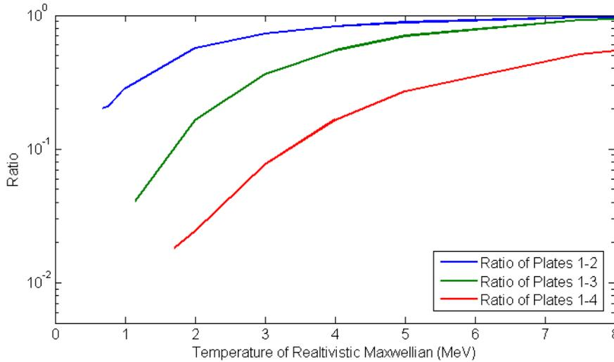
FIGURE 3. The ratios of layer 1 to each sequential layer for the total energy absorbed by the image plate as a function of temperature.
