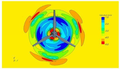
Figure 11a: Flow Field on the Pitot plane: Existing 50 kW ,  $Re=1.53x10^6$
