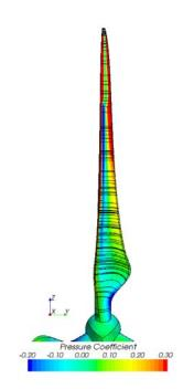
Figure 13a: Pressure coefficient on lower sides of the blade: 60 kW WT, Re=1.54x10<sup>6</sup>
