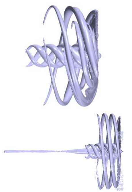
**Figure 12:** Vortical structures downstream the wind turbine (central and tip vortex) a) Existing 50 kW WT, Re=1.53x10<sup>6</sup>; b) 60 kW WT, Re=1.54x10<sup>6</sup>
