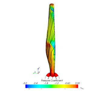
Figure 13c:Pressure coefficient on the upper side of the Existing 50kW blade, Re= $1.53 \times 10^6$
