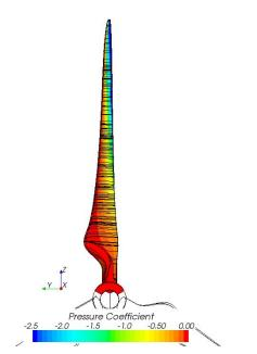
Figure 13b: Pressure coefficient on upper side of the blade: 60 kW WT, Re=1.54x10<sup>6</sup>
