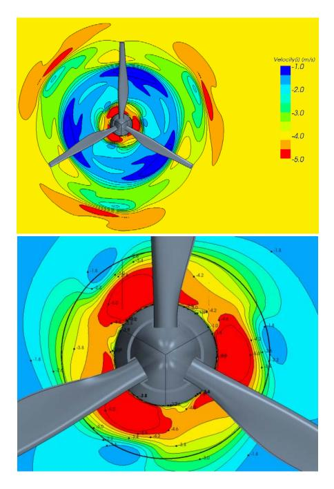
Figure 9: Flow Field on the Pitot plane ( $V_{wind}$  = 4.0 m/s,  $\Omega$  = 20 rpm)
