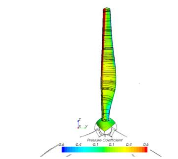
Figure 13d: Pressure coefficient on the lower side of the existing 50 kW blade, Re= $1.53 \times 10^6$
