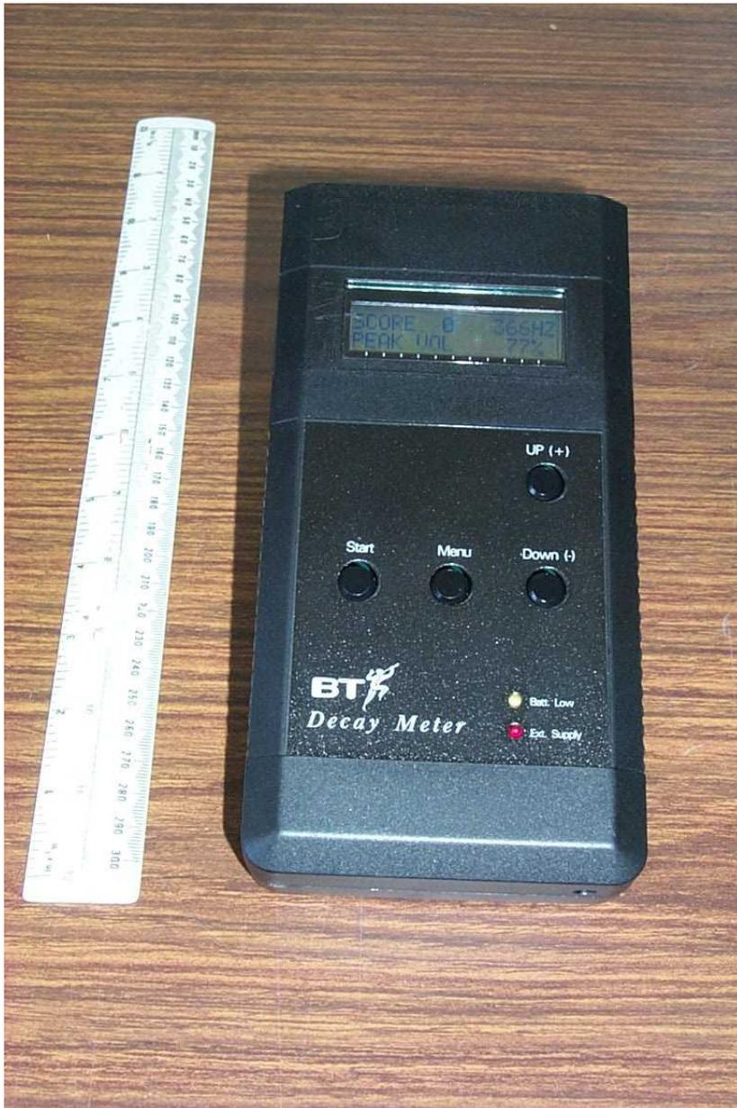
Figure 13 The pole decay meter.
