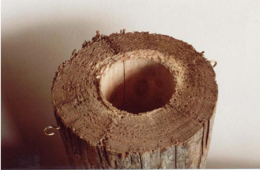
Figure 7 Short pole section showing cup hooks and 75 mm central “decay” hole.
