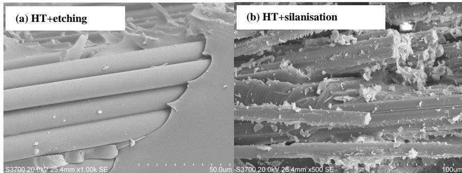
Figure 6 SEM photo of fractured area obtained from tested samples consisting of the CSM conditioned with (a) heat treatment at 500°C followed by HF etching and (b) the same heat treatment followed by APS silanisation
