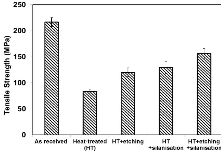
Figure 5 Tensile strength of CSM-epoxy composites with glass fibres received different treatments
