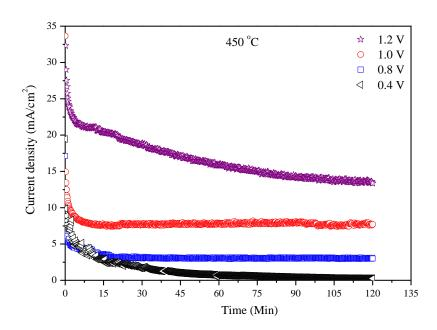
Fig. 6 Electrolytic cell performance stability at 450 °C and 0.4-1.2 V: The electrolytic cell was; wet H2, Ag-Pd|LiALO2-carbonate|Co3Mo3N-Ag, dry N2
