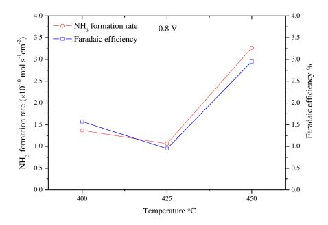
Fig. 5 Dependence of the rate of ammonia formation on the operating temperature. The electrolytic cell was; wet H2, Ag-Pd|LiALO2-carbonate|Co3Mo3N-Ag, dry N2
