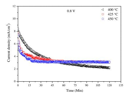
Fig. 3 Electrolytic cell performance stability at 400, 425 and 450  $^{\circ}$ C at 0.8 V: The electrolytic cell was; wet H<sub>2</sub>, Ag-Pd|LiALO<sub>2</sub>-carbonate|Co<sub>3</sub>Mo<sub>3</sub>N-Ag, dry N<sub>2</sub>.
