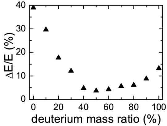
*Fig.5. Ion energy spread  $\Delta E / E$  as a function of the deuterium mass ratio in the composite DT targets at  $t = 100\tau$  from PIC simulations. The laser parameters are the same as in figure 1, and the total mass density of composite targets is fixed at  $\rho = 0.1 \text{ g cm}^{-3}$ .*
