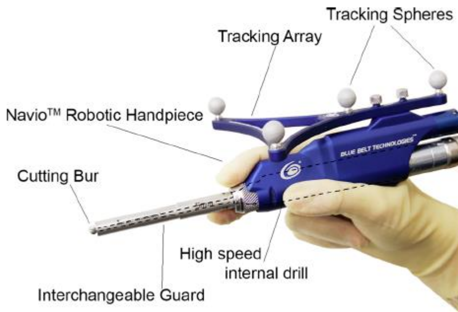
Fig. 1 The Navio™ hand piece includes a blue clamshell central unit for the user to grip, an array to allow it to be tracked by the system, and a metal guard covering the bur. Calibration of the bur to the end of the guard means that the system registers when the bur is covered by the guard or cutting.
