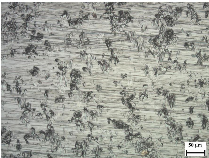
Figure 14. Outermost area (3) of the UNS S31600 after solid/liquid impingement.
