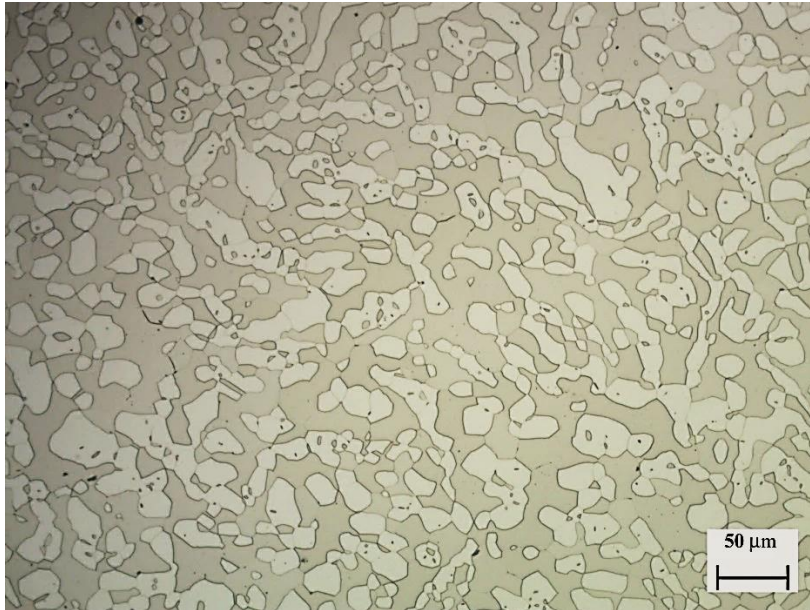
Figure 2. Ferrite matrix and austenite grains in UNS S32760
