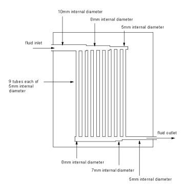
Figure 2: section through heat exchanger showing refrigerant ducts
