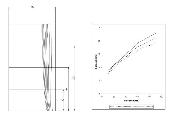
Figure 12: Ice profiles and ice thickness
