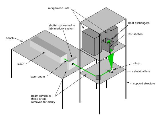
Figure 3: Diagram of experimental rig showing optical path.
