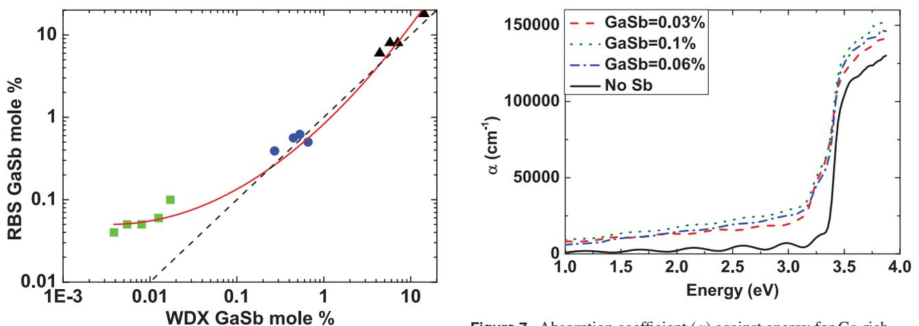
Figure 6. Comparison of the WDX and RBS technique's measurement of GaSb composition. Three sample series are shown including the Ga-rich (squares) and N-rich (circles) samples, as well as samples from Army research labs (ARL) which have a higher GaSb mole fraction (triangles). The solid line is a guide to the eye and the dashed line is the one to one correlation between RBS and WDX.
