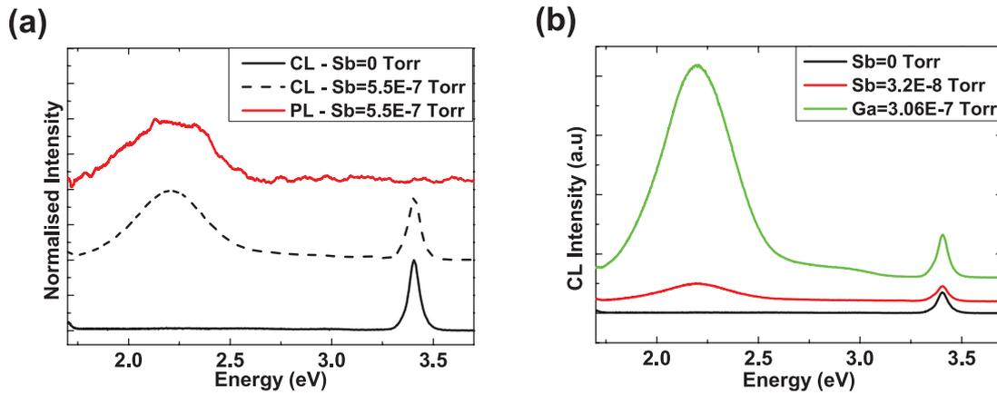
**Figure 8.** (a) Typical room temperature CL and PL spectra for samples with Ga flux =  $2.3 \times 10^{-7}$  Torr, with and without Sb and (b) room temperature CL spectra for samples with various Ga flux and fixed Sb flux =  $3 \times 10^{-8}$  Torr.
