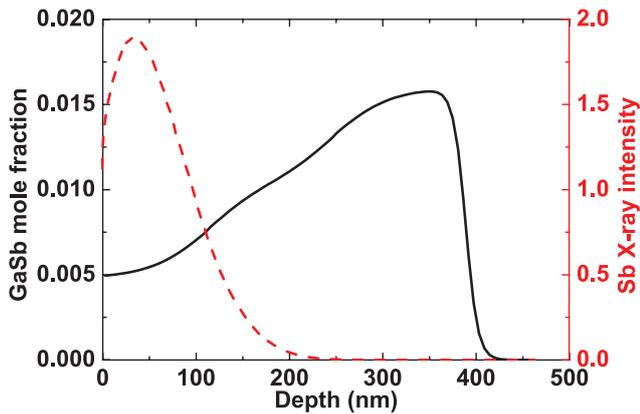
**Figure 2.** RBS measured depth profile of the GaSb mole fraction for a typical N-rich  $\text{GaN}_{1-x}\text{Sb}_x$  sample (solid line) and Monte–Carlo Sb x-ray generation with depth (dashed line).
