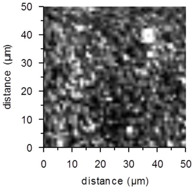
**Figure 10.** CL intensity map, showing the peak height in the range 2.0–2.4 eV, taken using an 8 kV, 10 nA, focussed beam for a sample containing Sb.
