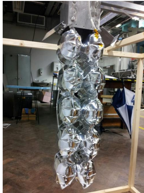
Figure 7: Prototype of 5x2cell deployed inflatable smart structure
