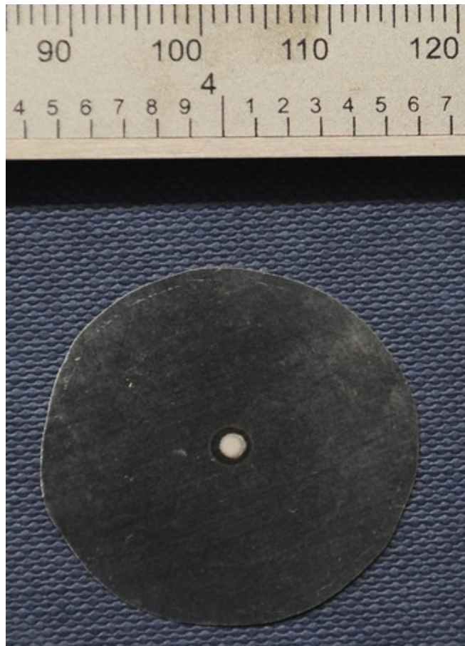
FIG. 3. Molybdenum target for X-ray generation showing the beam spot.
