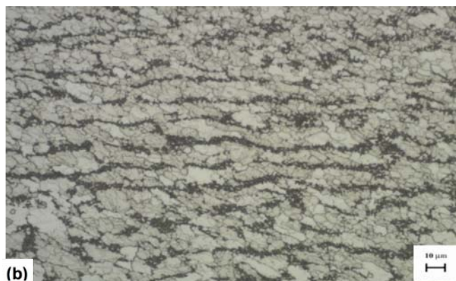
Fig. 5 TMAZ of (a) underwater FSW plate and (b) air FSW plate
