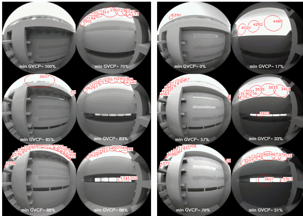
Figure 7: Atria design issues – visual comfort under advanced diffusing (left) vs. normal (right) roof glazing system.
