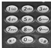
Figure 2: Nokia 5110 ISO standard 9-key keypad
