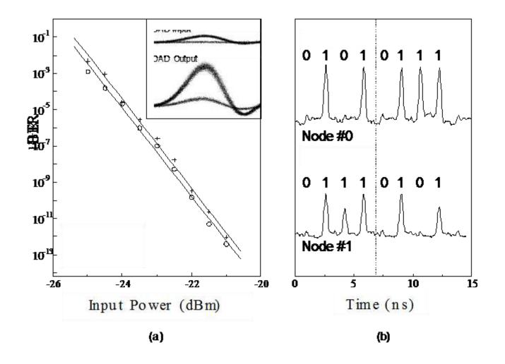
Fig. 4 BER of channels 0 and 1 against average single channel input power, and demonstration of rapid channel selection on bandwidth limited analogue detector*a)* BER of channels 0 and 1 against average single channel input power
