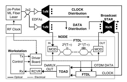
Fig. 2 Experimental OTDM computer interconnect and node architecture
