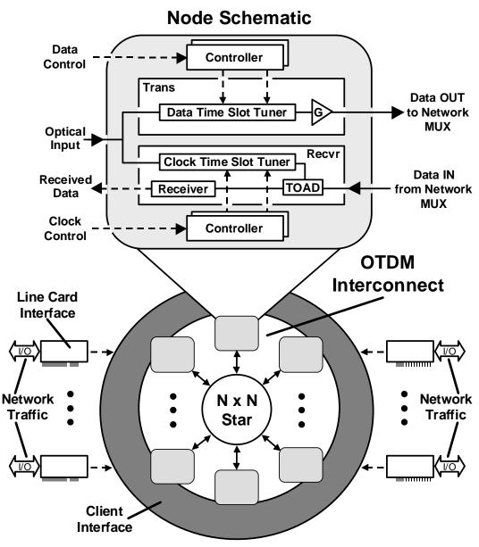
Fig. 1 OTDM router and node architecture
