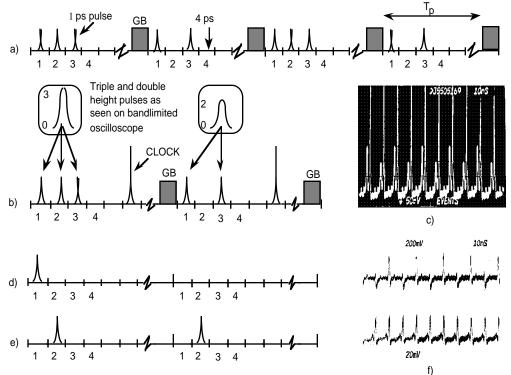
Fig. 4. Timing diagram. a) Two optically compressed packet headers "111" and "101<sup>''</sup>; b) Polarization multiplexed packets and clock; c) Oscilloscope trace of b); d) TOAD1 output after demultiplexig address bit 1; e) TOAD2 output after demultiplexing bit 2; f) Oscilloscope trace of d) and e).
