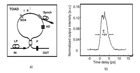
Fig. 1. a) TOAD diagram; b) 4 ps switching window
