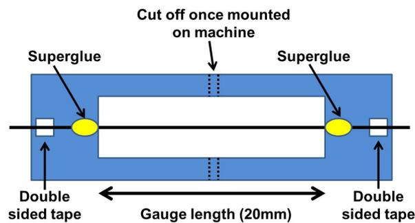
**Figure 1.** Schematic diagram of tensile sample preparation.
