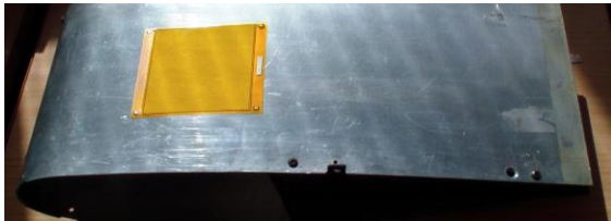
Figure 9 A piezoelectric patch on a test fin
