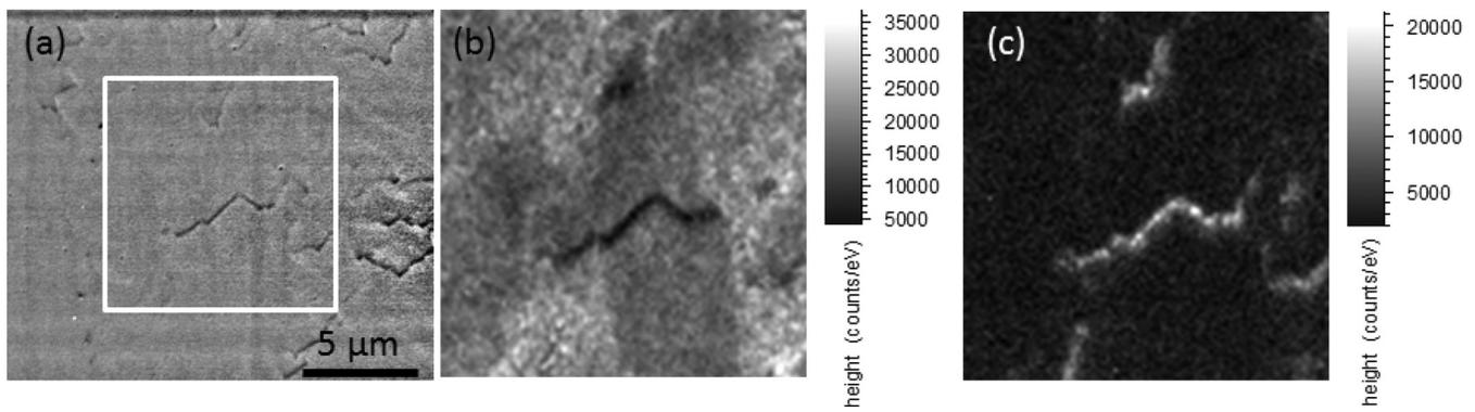
FIG. 3. SE image (a) and fitted  $10 \times 10 \mu\text{m}^2$  CL intensity maps of the 4.54 eV peak (b) and the 4.41 eV peak (c) of sample B.
