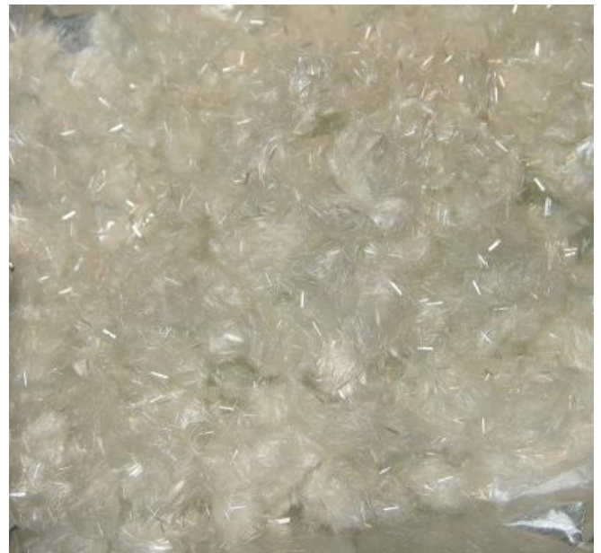
Figure 4. Glass fibres heat treated at 600°C taken from the barrel of the extruder
