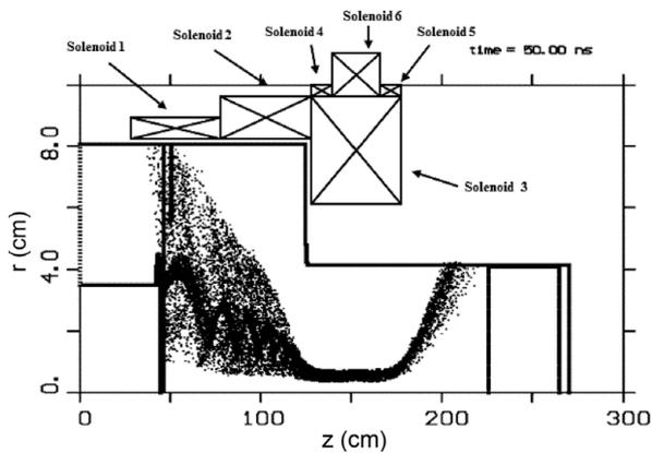
**Figure 1.** Experimentally consistent, waveguide-bounded PiC simulation geometry.
