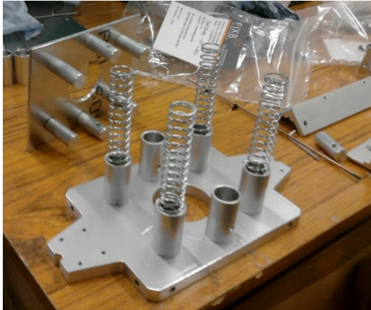
Figure 3: Base Plate Assembly with Retention Tubes
