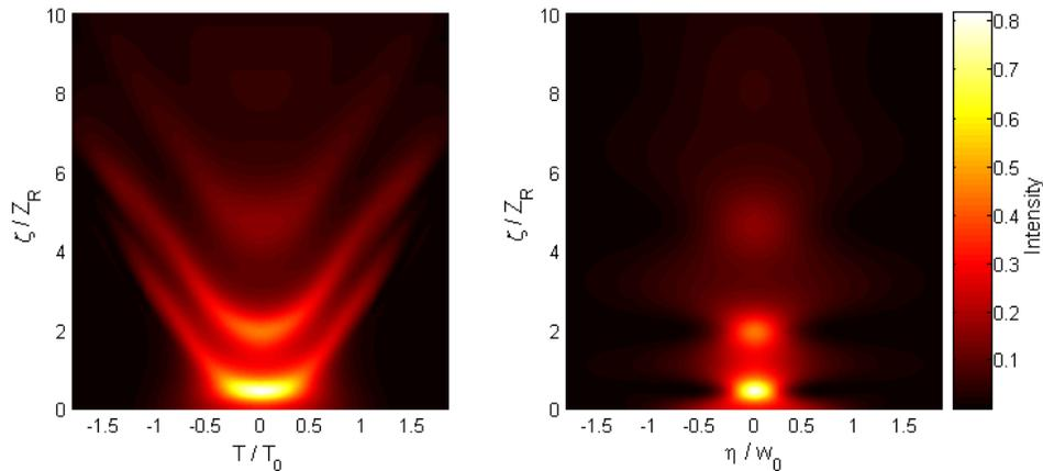
Fig. 12. Temporal (left) and spatial (right) evolution of a pulse in the normal GVD regime.  $\beta = +0.01$ ,  $\gamma = 15$ . Due to the spreading of the pulse along the temporal dimension, the power in the spatial slices is reduced to the point at which no self-focusing can occur, resulting in collapse of the pulse.
