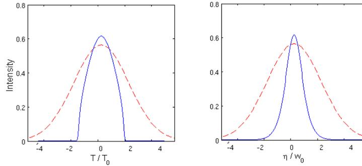
Fig. 11. Left - initial (red dash) and final (blue) temporal cross section. Right - initial and final spatial cross section. The pulse has narrowed in both dimensions during propagation, due to self-focusing in the spatial dimension, resulting in the  $\text{sech}^2$  distribution, but due to untrapped energy being shed in the temporal dimension, resulting in a parabolic profile.
