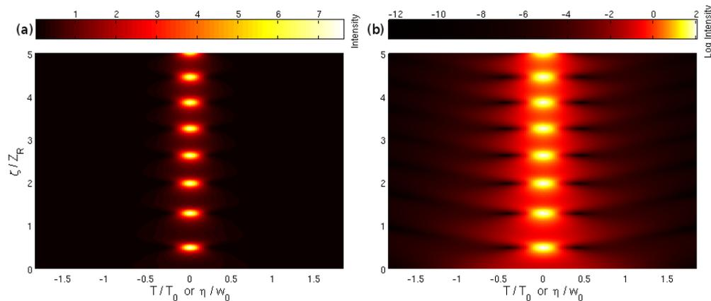
Fig. 13. (a) Evolution of the T/X profile in the anomalous-GVD regime.  $\beta = -1, \gamma = 20$ , Saturating nonlinearity. (b) Logarithmic intensity scale of (a). The results are similar to 2D spatial propagation of the pulse with a spatial dimension replaced with the temporal one
