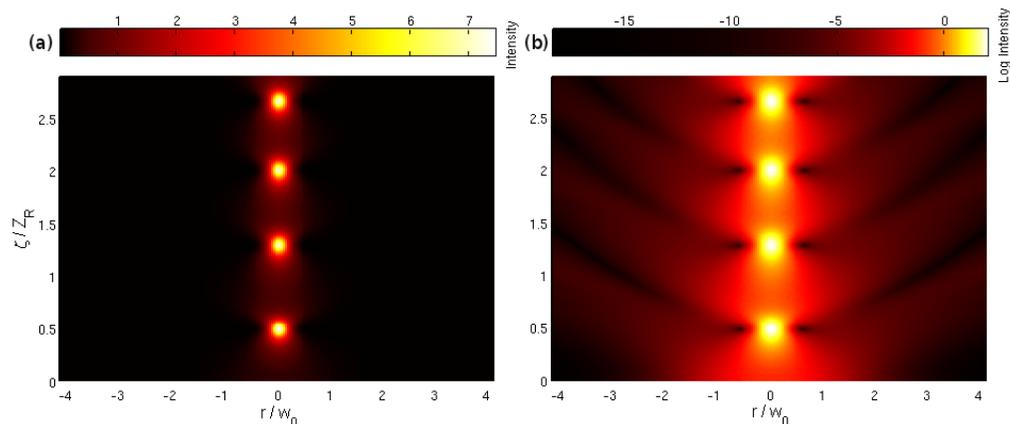
Fig. 7. (a) Oscillations in a 2D cw beam propagating in a saturable medium.  $r$  is the transverse radial variable. Intensities reached are roughly 6 times that of the 1D case.  $\gamma = 20$ ,  $\sigma = 0.1$ . (b) Logarithmic intensity scale of (a), showing shedding of low levels of energy during defocusing, reducing the power of the beam.
