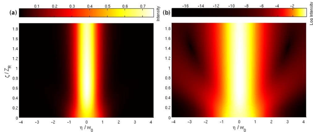
Fig. 1. (a) Reshaping of the self trapped beam from initially Gaussian input to a  $\text{sech}^2$  distribution. Energy is shed and oscillation in the amplitude is caused by the reshaping process,  $\gamma = 5.8$ . (b) Logarithmic intensity scale of (a), revealing the energy being shed upon entry to the medium.
