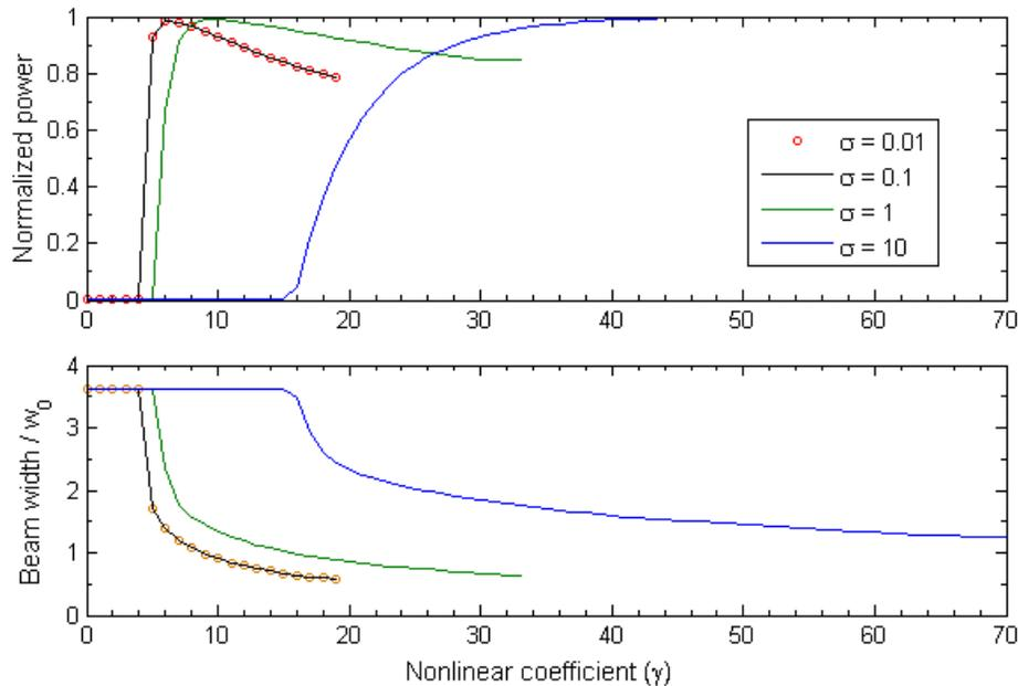
Fig. 6. Final power (top) and resulting beam width (bottom) dependence on the nonlinear coefficient for different values of  $\sigma$ . It can be seen that the point of self-trapping and hence the required critical power depends on the saturation parameter, requiring greater levels of power when there is greater saturation. At the point of exciting the second self-trapped state the solution becomes unstable and symmetry breaking instabilities occur.
