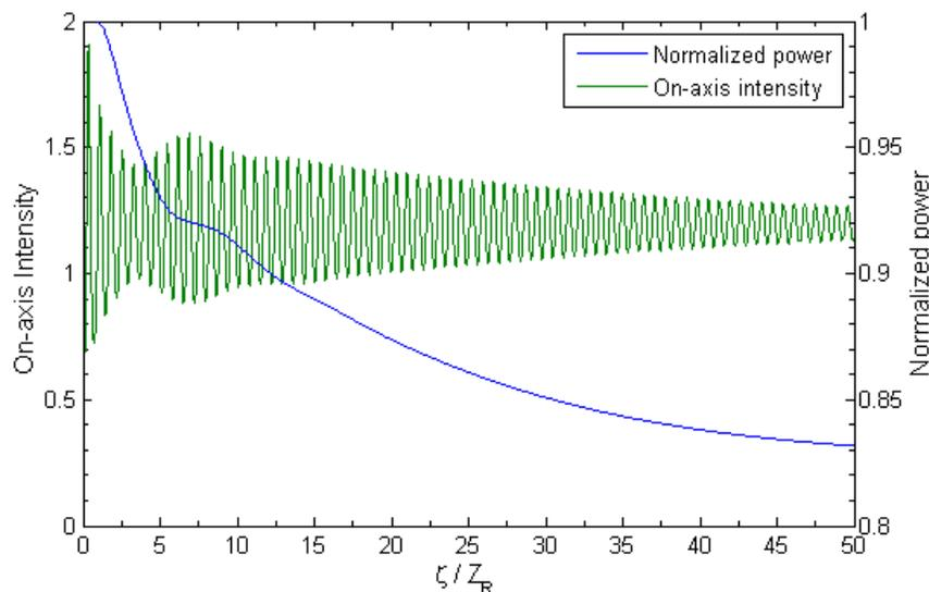
Fig. 3. Intensity (green) and normalized power (blue) for saturating NLS propagating  $50 Z_R$ .  $\gamma = 16$ ,  $\sigma = 0.1$ . Here it can be seen that after the initial reshaping process there is a long lived damped oscillation in the amplitude rather than the stable soliton solution of the cubic NLS, and loss of power during propagation that is proportional to the oscillation in the width and amplitude.
