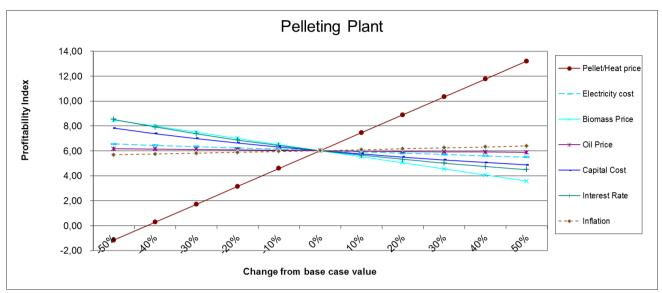
Figure 3. Sensitivity analysis for the pelleting plant
