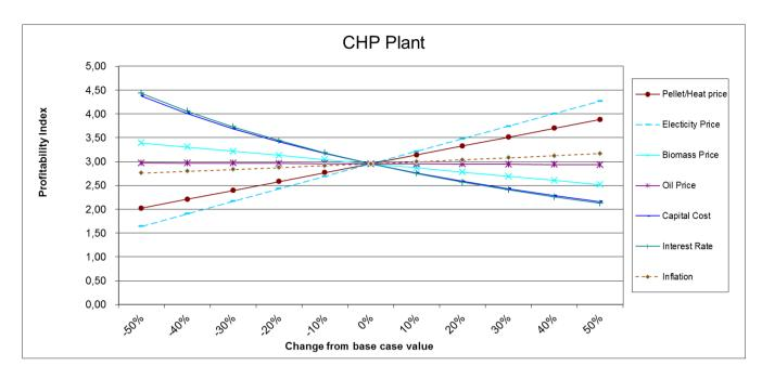
Figure 4. Sensitivity analysis for the CHP plant
