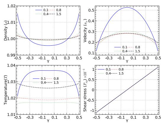
Fig. 7. Simulation results of the ES-BGK model applied to force-driven Poiseuille flow at various Knudsen numbers (labeled) and for  $g_x = 0.22$ .
