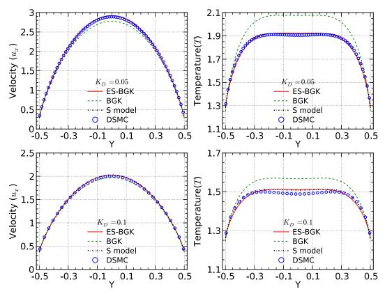
**Fig. 2.** Velocity and temperature profiles of force-driven Poiseuille flows for  $K_D = 0.05, 0.1$  with  $g_x = 1$ . Hard sphere molecular interactions are considered, i.e.  $\omega = 0.5$ . The solid lines are the ES-BGK data with Pr = 2/3 and the symbols are the DSMC data. The BGK data (dashed lines) and the S-model data (dashed-dotted lines) are also included.
