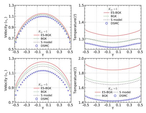
**Fig. 3.** Velocity and temperature profiles of force-driven Poiseuille flows for  $K_D=1,5$  with  $g_x=1$ . Hard sphere molecular interactions are considered, i.e.  $\omega=0.5$ . The solid lines are the ES-BGK data with Pr=2/3 and the symbols are the DSMC data. The BGK data (dashed lines) and the S-model data (dashed-dotted lines) are also included.
