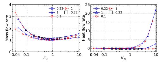
**Fig. 9.** Mass and heat flow rates predicted by the ES-BGK model (the solid lines with circles and upper triangles), the Boltzmann equation (the squares) and the BGK model (the dashed lines with hexagons and right triangles). The body force magnitudes are presented in the legend. The BGK data are from Table 2 of Aoki et al. [20], with the Knudsen numbers converted to  $K_D$  accordingly. The mass and heat flow rates are further normalized by the corresponding body force magnitude.
