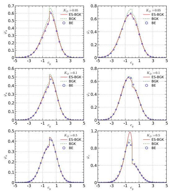
Fig. 5. Comparisons of BGK and ES-BGK marginal distribution functions  $\varphi_a$  and  $\varphi_c$  at the left wall boundary (y=-0.5) with those of the Boltzmann equation (BE) for  $g_x=1$ .
