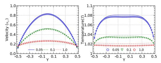
**Fig. 4.** Velocity and temperature profiles of force-driven Poiseuille flows with  $g_x = 0.22$ . Hard sphere molecular interactions are considered, i.e.  $\omega = 0.5$ . The lines are the ES-BGK data with Pr = 2/3 and the symbols are the DSMC data. The Knudsen numbers are  $K_D = 0.05, 0.1$  and 1.0 as noted and they are distinguished by different plot styles as shown.
