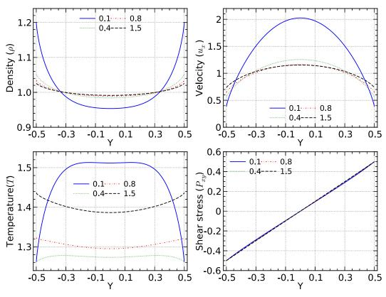
Fig. 8. Simulation results of the ES-BGK model applied to force-driven Poiseuille flow at for various Knudsen numbers (labeled) and for  $g_x = 1$ .
