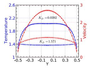
**Fig. 1.** Convergence analysis: the present results (lines) are compared with the BGK data (symbols) reported by Aoki et al. [20]. Maxwell gas interactions are used in both models, and the results are comparable by letting b=0,  $\omega=1$  in the ES-BGK model. Two Knudsen numbers 0.0392 (the upper lines and symbols) and 1.571 (the lower lines and symbols) are considered. The agreement between the two set of results confirms the validity of our chosen molecular velocity and spatial grids.
