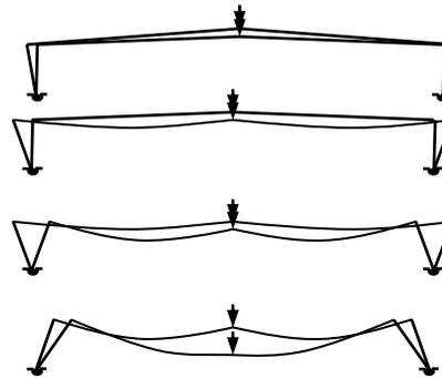
Fig. 1. Snap-through mechanism
