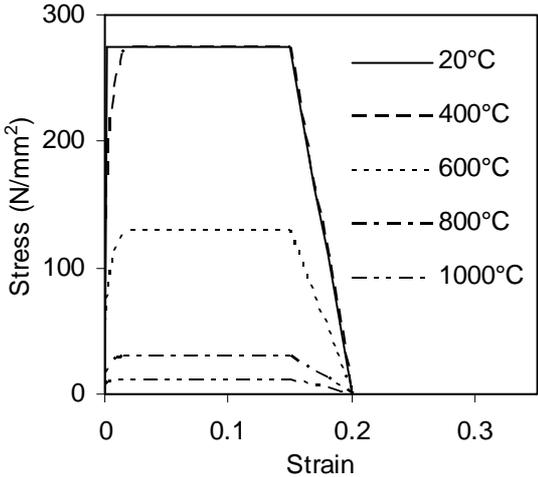
Fig. 3. Stress-strain curves for steel grade S275
