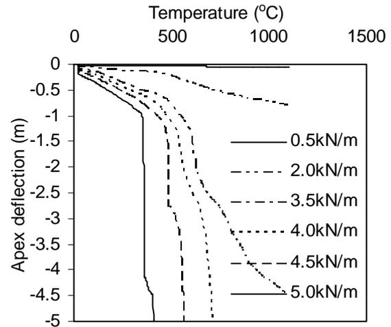
Fig. 14. Effect of different vertical loads
