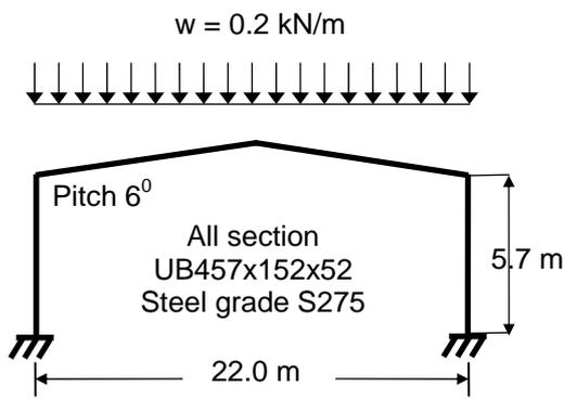
Fig.10. Details of exemplar single span portal frame after SCI (Ref. 1)
