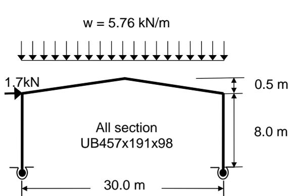
Fig. 5. Details of single span frame after Song *et al* (Ref.2)
