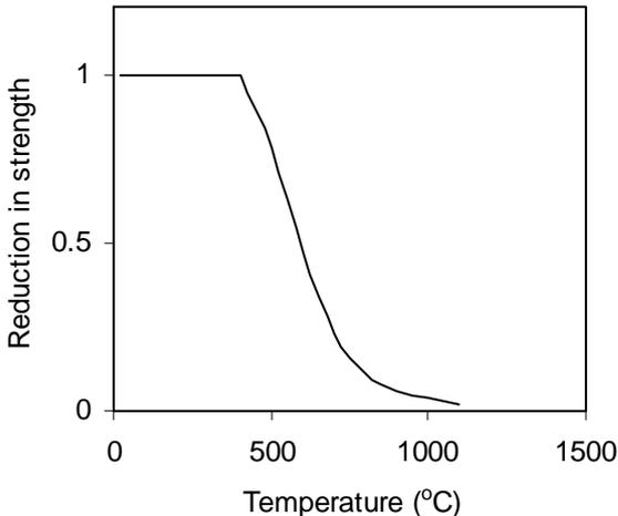
Fig.2. Variation of reduction in ultimate strength of steel against temperature
