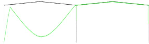
Fig. 8 Deformed shape at 1100°C (Deflections magnified by a factor of 50)
