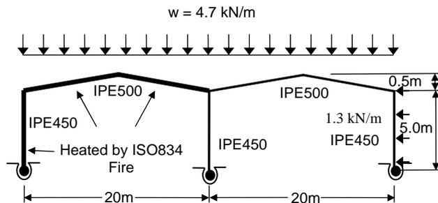
Fig.7. Details of double span frame after Vassart et al (Ref.5)
