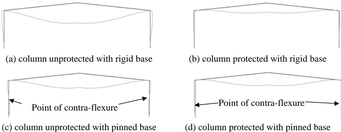
Fig. 12 Deformed shape (Deflection magnified by a factor of 25)
