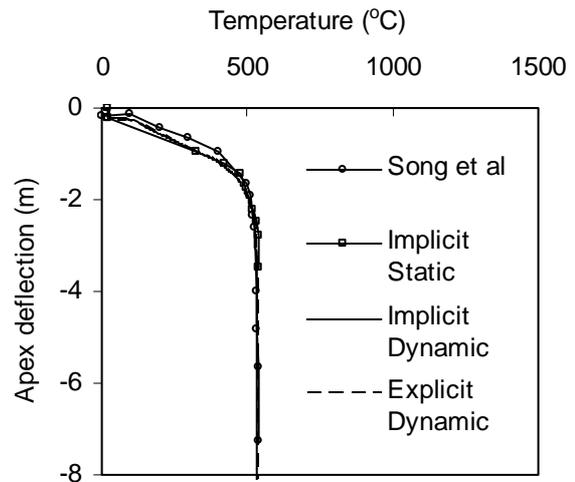
Fig. 6. Variation of apex deflection against temperature for single span frame
