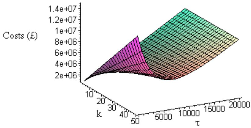
Figure 6 Total cost plane as a function of test time and  $k$
