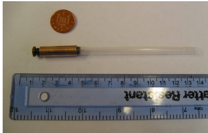
Figure 3.2: (a) Diagram and (b) photo of pressure cell for the SQUID.
