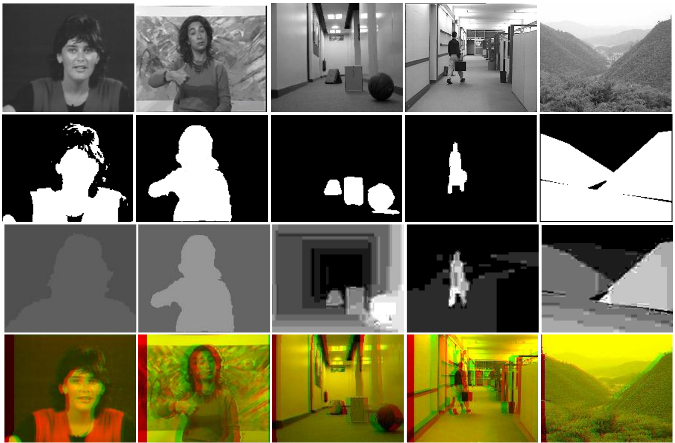
Fig. 7: Results extracted from five test sequences including “Miss America”, “silence”, “Aisle1”, “Hall monitor”, and “Mountain” (from left to right). From top to bottom, four rows respectively correspond to original image, segmented results, estimated depth maps, and synthesized stereo image.
