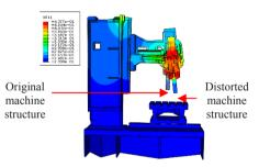
Fig. 4. Simulated visual representation of deformation of the machine due to internal heating
