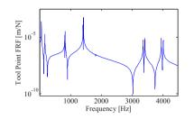
Fig. 4. Tool point FRFs at 30 000 rpm for stiffer connection
