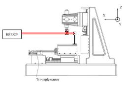
Fig. 7. Experimental setup for positioning test
