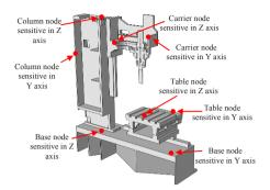
Fig. 7. Environmental sensitive nodes within the full machine
