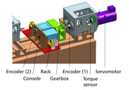
Fig. 5. Picture of gear system measuring arrangement
