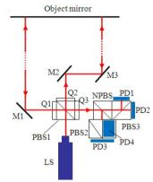
Fig. 3. Optical configuration of angle interferometer
