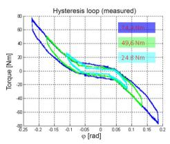
Fig. 6. Measured hysteresis loops of the gear system
