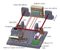
Fig. 5. The integrated structure of a three-angle sensor
