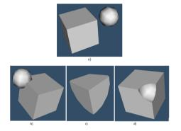
Fig. 4 The regular cube and cursor: (a) source objects, (b) union, (c) intersection and (d) difference.
