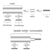
Fig. 2. Spindle Holder Tool assembly
