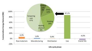
Fig. 3. Environmental Profile of an injection moulding machine [2]
