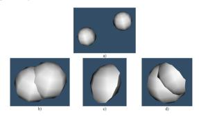
Fig. 3 Objects for the case 1: (a) source objects, (b) union, (c) intersection and (d) difference.
