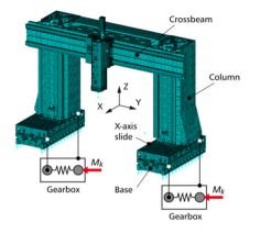
Fig. 8. FE model of the machine and the connection with simplified models of the X-axis gear system
