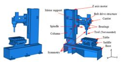
Fig. 1. Generated CAD model of the machine assembly
